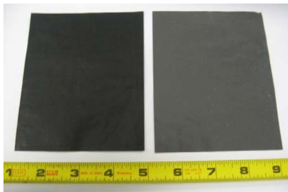
Fig.1. two samples of paper-like nanocarbon sheet created through our Nano to Marco™ manufacturing process. Final properties depend on the type of nanocarbons used as raw materials and on the chosen manufacturing process steps (measuring tape in inches).
